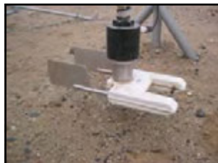
Sand Particle Counter (30 to 600 \mu\text{m} )
