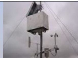
Dust emission OPC (0.3 to 7 \mu\text{m} )
