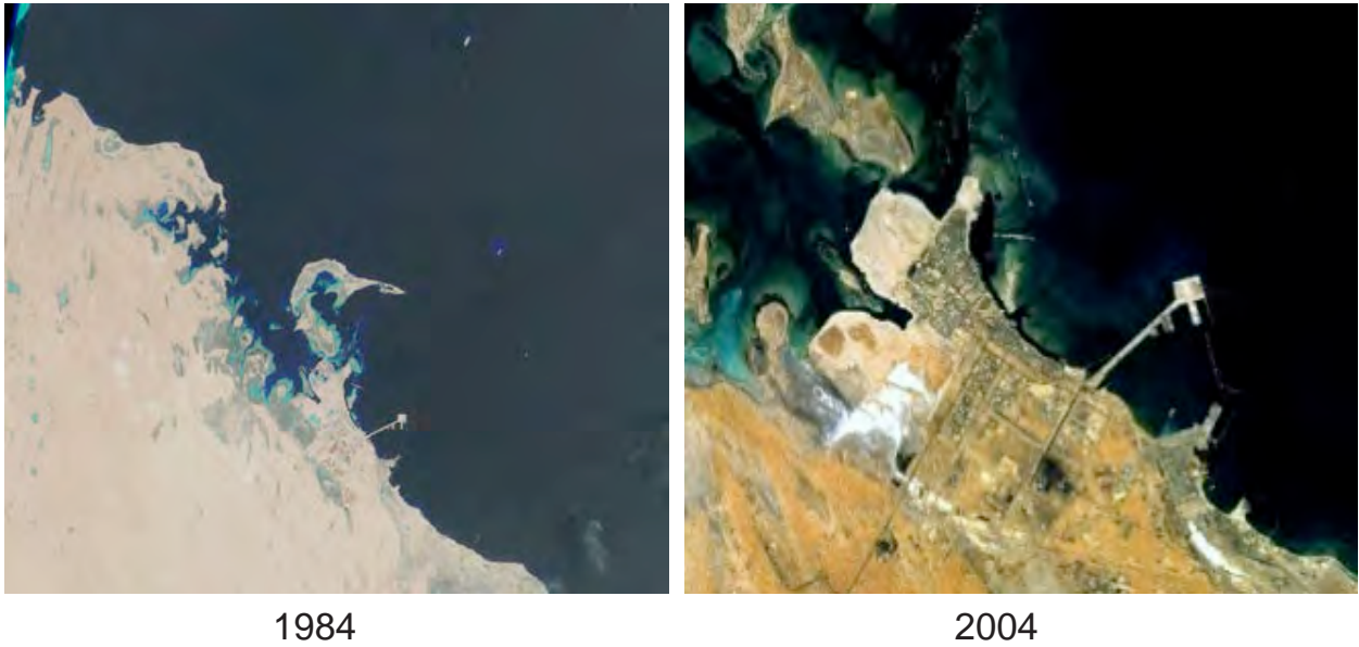
Figure 14. Industrial development in Jubail. (In Saudi Arabia, approximately 40% of the coastal area on the RSA has been developed into industrial and supportive residential and commercial areas along the coast. Particularly Jubail, Tarut Bay, Dammam and Khobar, demonstrate the extent of coastal infilling and landfilling in the Region. In Jubail city, more than 200 million cubic meters of sediments adjacent to the development have been removed and 46.5 square km of coastal habitat have been dredged in Jubail and Dammam. These areas of shallow subtidal coast are highly productive and form nursery and feeding grounds for most commercial shrimp and fish species).
